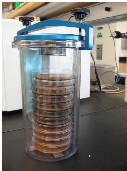
Figure 4: Gradient plates in the jar providing a microaerophilic environment using BBL Campypak Plus microaerophilic system envelopes.
