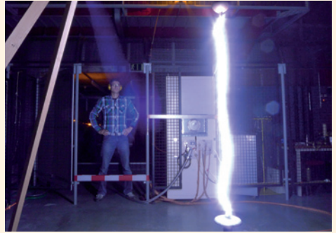
Figure 1. A large spark is generated in a laboratory at the Technical University of Eindhoven, the Netherlands. Experiments with sparks are used to study X-ray and gamma-ray photons from relativistic electrons, accelerated in the electric field of sparks and natural lightning. The photons are “bremsstrahlung” from the interaction of the electrons with the air. Bursts of gamma radiation are observed from satellite above thunderstorms. The precise source mechanism is unknown.
