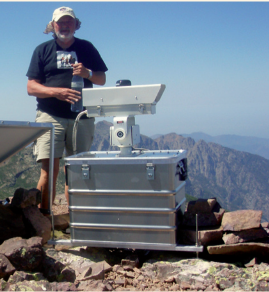
Figure 2. An optical imaging system for observation of sprites, the electric discharges in the mesosphere above thunderstorms. The system is located on Mount Corona in Corsica and can observe the atmosphere above thunderstorms reaching from Spain in the West, over Southern France in the North and to Italy in the East. It has its own power system and is controlled via a satellite link.
