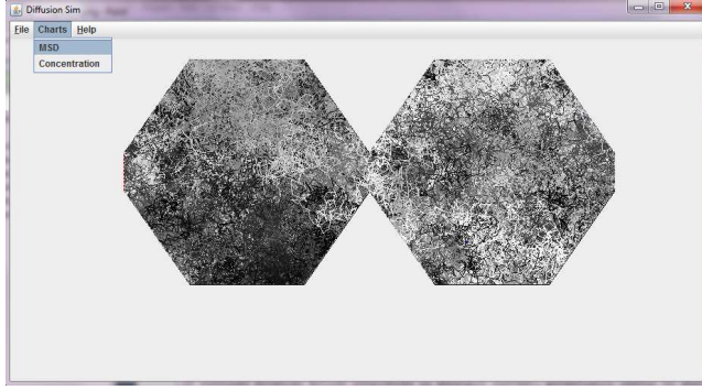
Figure 2: Two containers with big channels between them. 400 particles move randomly inside them drawing lines from light (early stage of moves) to dark (later stage of moves) color.
