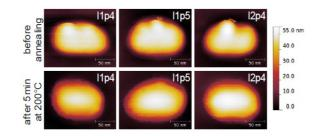
Fig.1: Atomic force micrographs of three individual gold nano-rods, as deposited (top row) and annealed (bottom row). The somewhat broader appearance of the annealed rods is attributed to a tip-artifact.
