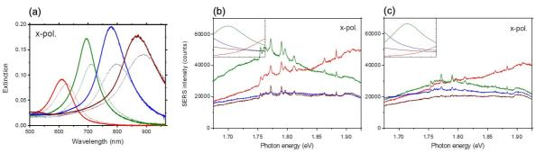
Fig. 2: Exitnction spectra (a) of gold nano-rod arrays, and corresponding SERS-spectra before (b) and after (c) annealing with rhodamine 6G.
