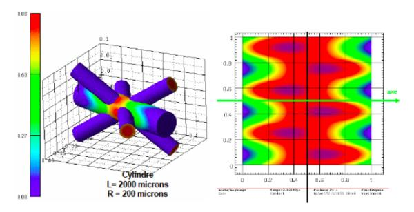
Fig. 1: degree of uniformity of laser irradiation on a cylindrical target (calculations with the Code Ceclad by Gabriel, J.-L.Feugeas, and Ph.Nicolai of CELIA)
