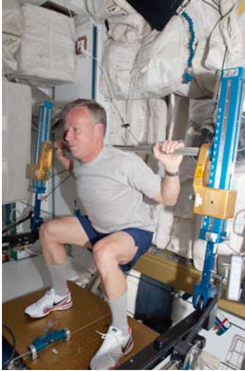
Figure 5: NASA Astronaut Steve Lindsey using the advanced Resistive Exercise Device (aRED), providing high loads to weight-bearing bones (Credit: NASA)
