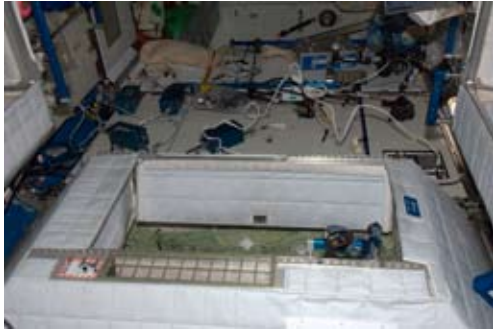
Figure 14: Sleeping cabins on-board the ISS are built into the floor, walls and ceiling, providing astronauts with privacy and a fixed place to sleep (Credit: ESA/NASA)
