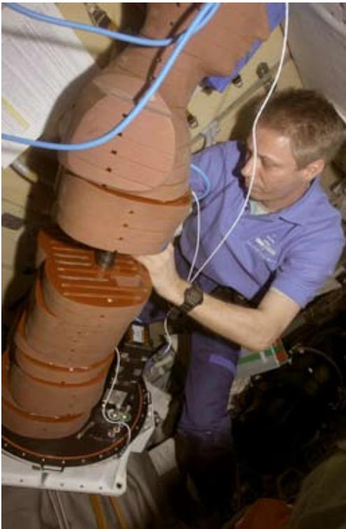
**Figure 6:** ESA astronaut Thomas Reiter sets up the MATROSHKA phantom on the ISS (Credit: NASA).
