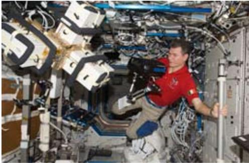
**Figure 4:** Figure 4: ESA astronaut Paolo Nespoli installing ALTEA hardware for the ALTEAshield-survey experiment, aimed at performing a 3D survey of the radiation environment in the US Laboratory of the ISS. (Credit: NASA).
