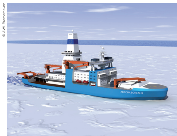
Figure 11. The Aurora Borealis icebreaker was endorsed by the European Polar Board in early 2000. The vessel provides unique capacities to carry out interdisciplinary research in almost 90% of polar waters in any season and weather conditions. The model underwent severe tests for both frontal and lateral ice-breaking capabilities in Hamburg and in Finland at the Aker Arctic's towing tank.
