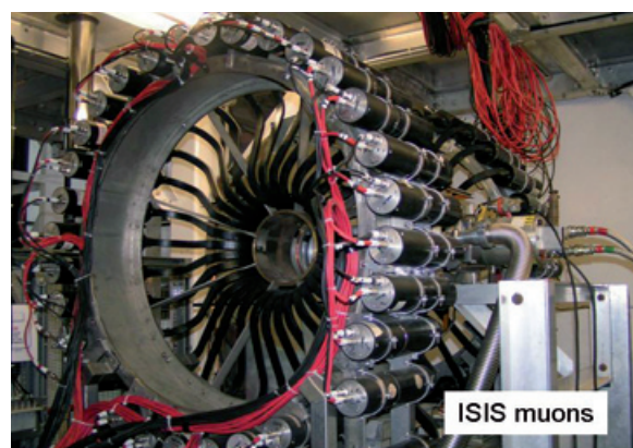
ISIS muon spectrometer. The detectors (black) trace the positrons emitted after the desintegration of muons implanted in the studied materials. Magnetism can hence be explored at the atomic scale down to 40 mK.
