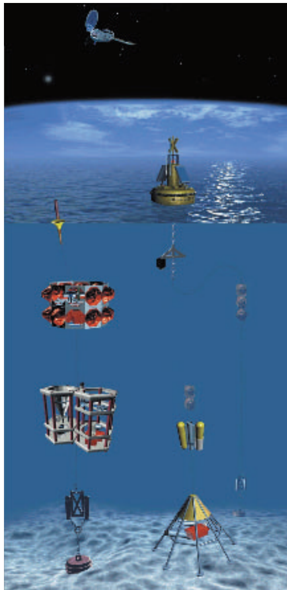
The DOMEST system for observing material transport at the sea bed includes traps, video, profiling CTD and other sensors, with acoustic and satellite retrieval of data using bi-directional communication
