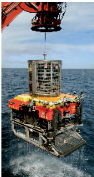
Deployment of Isis deep ocean ROV
