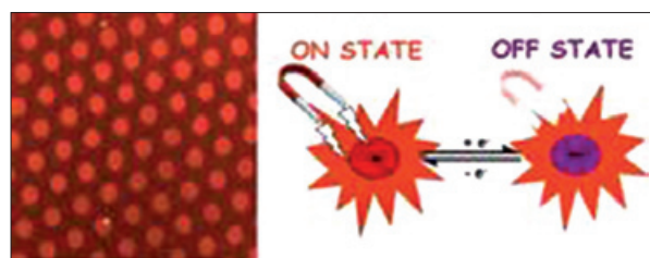
Confocal microscope image of a self-assembled monolayer of a polychlorotriphenyl methyl radical patterned on a quartz surface. This multifunctional molecule behaves as an electroactive switch with optical and magnetic response.
