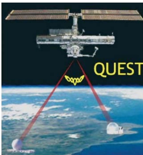
Figure 5.5. The QUEST proposal. The source for entangled photons is placed for example on the ISS, and the two photons are sent to two separate ground stations. The objectives of this experiment are to demonstrate, for the first time in space: (1) absolute secure global distribution of cryptographic keys from space, based on novel quantum communication techniques, and (2) fundamental quantum physics principles beyond the capabilities of Earth-bound laboratories by using the added value of space environment.
