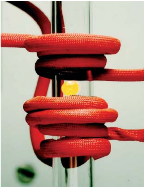
Figure 5.13: Levitation processing of a liquid metallic sample in 1g, resulting in a non-spherical geometry.
