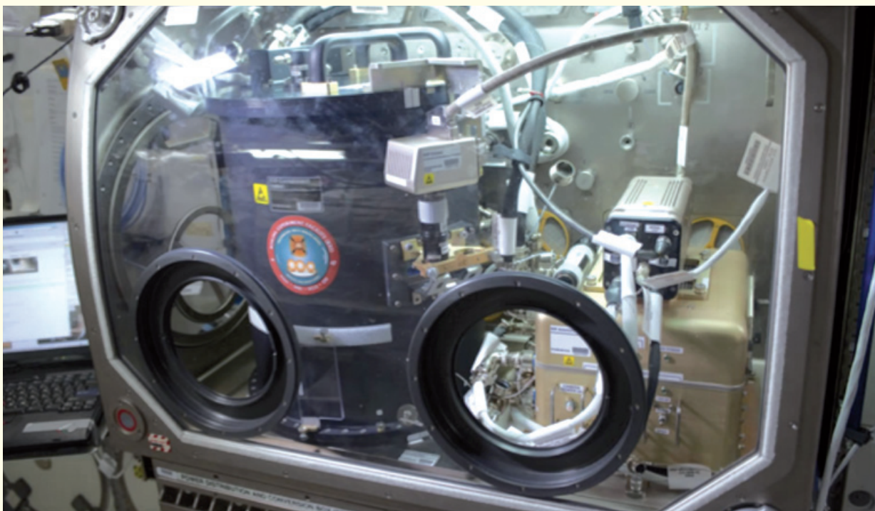
Figure 21: The boiling experiment facility installed inside the microgravity science glovebox on-board the ISS (Credit: NASA)
