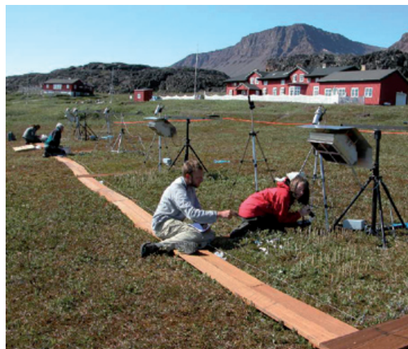
Infrared heating systems to study the effects of climate warming on tundra ecosystems
