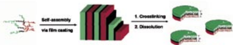
Figure 1: Schematic synthesis of Janus discs, based on the selective crosslinking of PB domains of a SBT terpolymer with lamella-lamella (ll) morphology.
