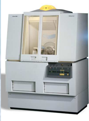
Powder diffractometer Xpert-Pro Panalytical Configuration \Theta - \Theta (Collaboration LDSMM , Y.Guinet, F. Capet)
