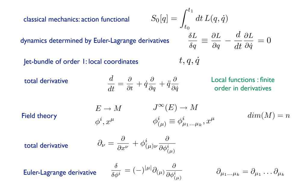
In the case of classical mechanics, the action becomes a functional, and the dynamics of the system is determined by the Euler-Lagrange equations, which are ordinary differential equations.
