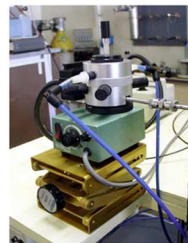
Liquid phase – Membrane inlet – Real-time online monitoring (H 2 , O 2 , CO 2 )
