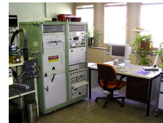
Liquid phase – Membrane inlet – Real-time online monitoring (H 2 , O 2 , CO 2 )
