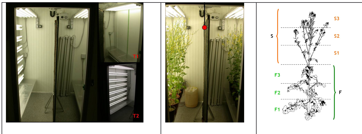
Fig. 1. Growth chamber equipped with two light levels: T1, conventional light source (from the top); T2, top and lateral light sources (left figure). Brassica c. subjected to two different radiation treatments (inner figure). Considered plant layers (right figure).
