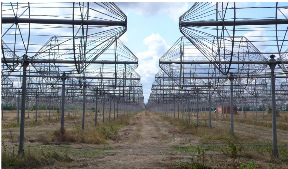
Fig. 20: The World's largest decameter array operated by the Institute of Radio Astronomy in Kharkov of the Ukrainian Academy of Sciences is used also for the search of radio signals originated in exoplanet magnetospheres and decametric type II bursts which are related to stellar CMEs.
