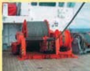
Seabed and deployment Winch
