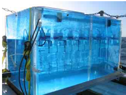
Shipboard chemostat system (D.A. Hutchins' prototype)
