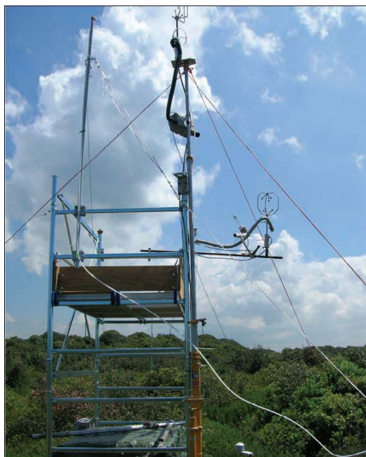
A tower to measure VOC fluxes at a field campaign in Castelporziano, Rome (photo: Francesco Loreto)
