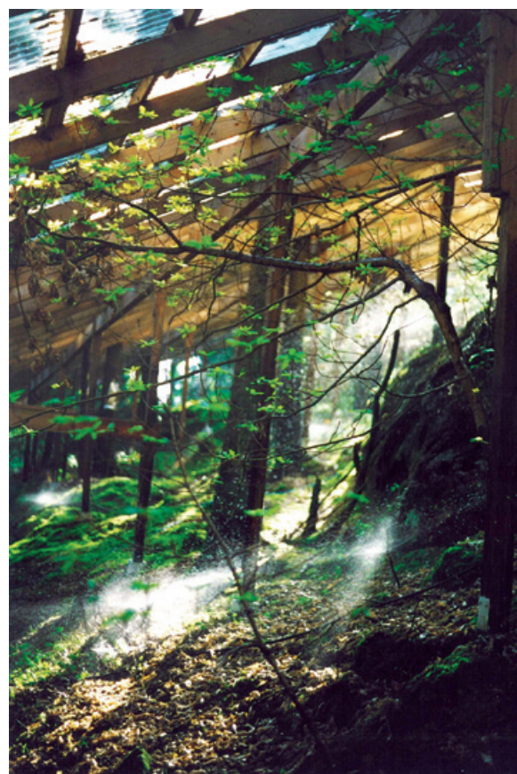
Manipulation of precipitation and N deposition at the roof project at Gårdsjön in Sweden.
