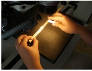
Figure 2. Use of a piece of chalk to identify difficult rings, during the measurement process (left). Detail of one dated core, with the dots system to locate the calendar year (right).
