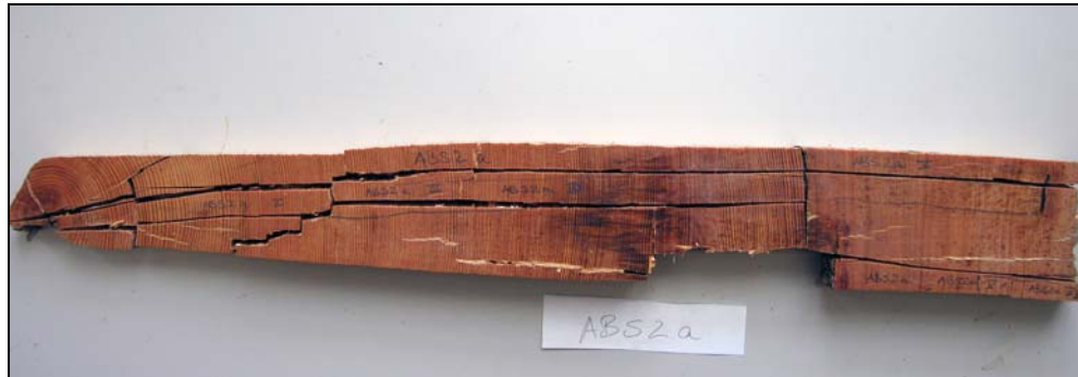
Figure 1: Several fragments of disc No. ABS2a that are used for the MXD measurements in their correct order.
