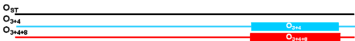
Fig. 7: Diagram of the three arrangements studied. The boxes indicate the region that it is inverted in relation with the standard arrangement.
