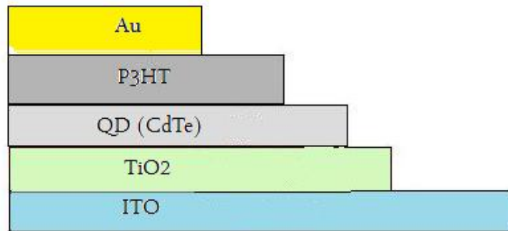
Figure 9: The scheme of solar cells consisting of CdTe nanoparticles
