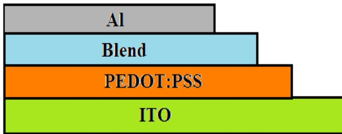
**Figure 7.** The scheme of the solar cell
