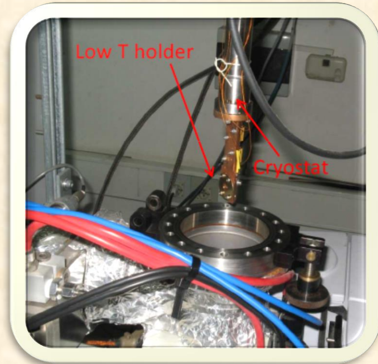
Picture of the cold finger with the MgF_2 window used as substrate
