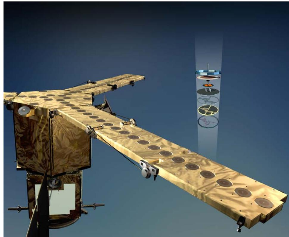
Interferometric Radiometer Antenna Arms
