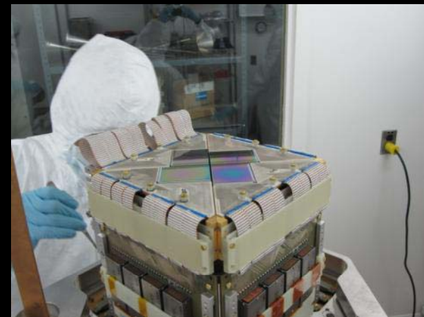
SCUBA2: Arrays of Transition Edge Superconducting Devices
