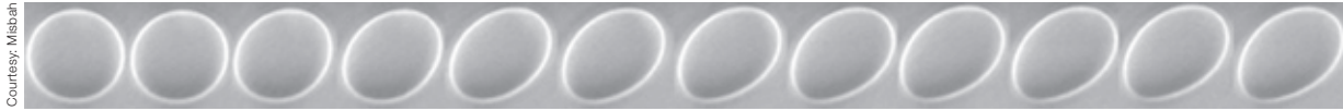
Figure 2.3.1.7: The effect of shear flow in vesicles (model of blood cells) flowing in a pipe under weightlessness.
