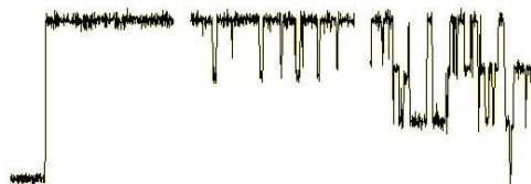
Figure 1: Black-lipid Membrane experiment : blockage of a single maltoporin trimer in presence of various concentrations of maltohexaose.
