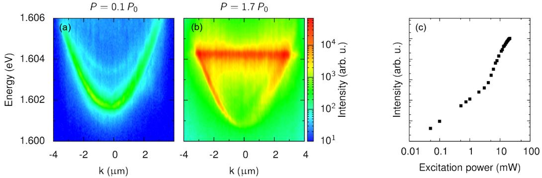
Fig. 1: Exciton-polariton dispersion below (a) and above (b) the threshold for polariton condensation. (c) Emission intensity as a function of the exciton power.
