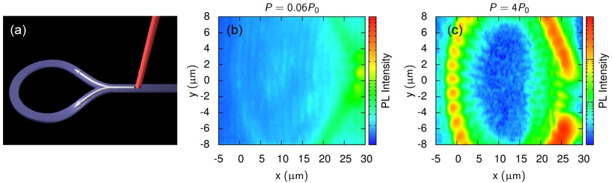
Fig. 2: Schematic of the structure where the red line represents the excitation laser whereas the white arrows indicate the flow of the polaritons. The real space image of the ring part of the structure below (b) and above (c) the threshold.
