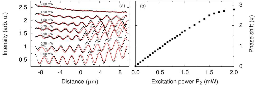
Fig. 3: (a) Intensity pattern in the ring part of the half interferometer structure for different excitation powers  $P_2$ . The excitation power for the creation of the condensate was kept constant to be  $P_1 = 16$  mW. The symbols denotes the intensity obtained from the experiment whereas the red solid represents the calculated interference pattern as explained in the text. (b) The extracted phase difference between the anti- and clockwise propagating condensate as a function of  $P_2$ .
