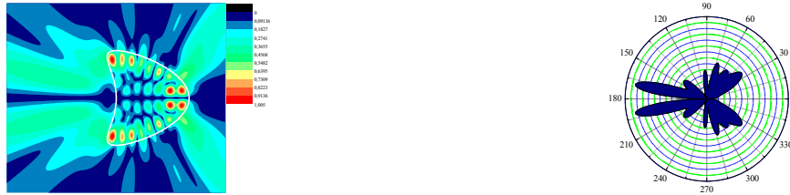
Fig. 4. The same as in Fig. 3. Horse-shoe like mode is an odd one with \kappa = 9.0652 , \gamma = 8.1136 \cdot 10^{-2} , D = 5.65 . Other parameters are N = 50 , \alpha = 1.5 .
