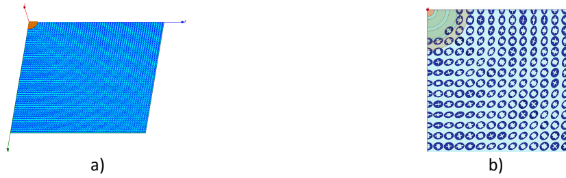
Fig.10 Main view of the complete implemented MTS, composed by elliptical pixels with cross type hole inside. a) Top View. b) Zoom out of the center.
