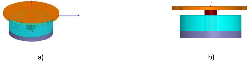
Fig.3 Details of the employed feeding system: circular waveguide providing TE 11 excitation mode with corrugated hat on top. a) Top View b) Lateral View
