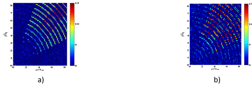
Fig.10 Implementation error (%) predictable at the implementation of the MTS with pixels for a) TM mode b) TE mode.
