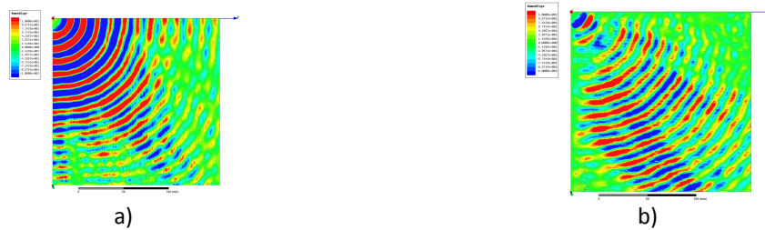
Fig. 11 Copolar (a) and Crosspolar (b) component of the field close to the aperture at 13GHz.
