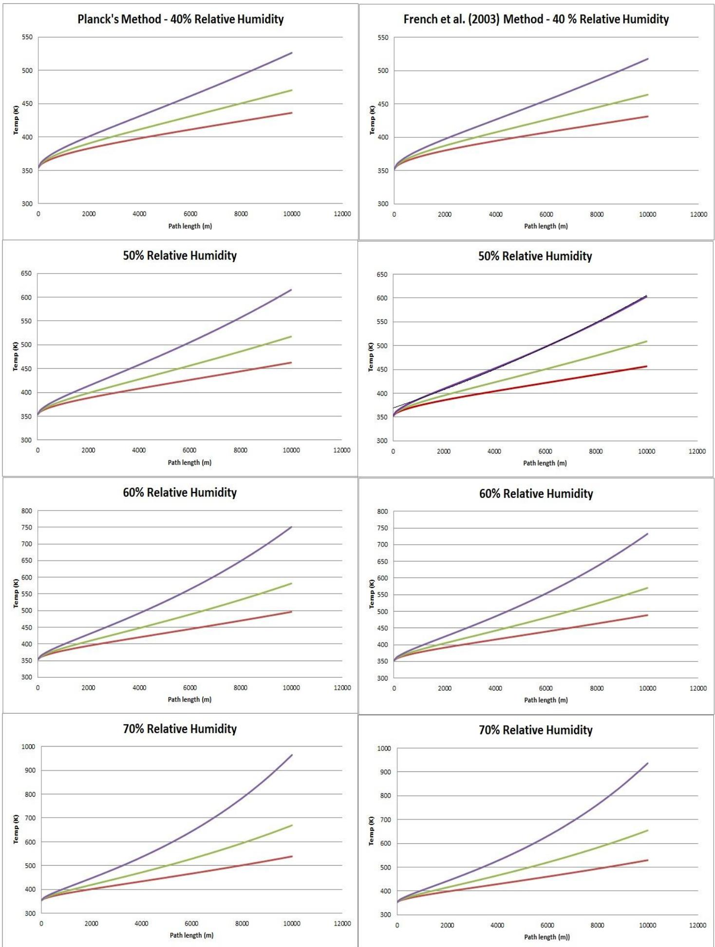
Figure 2 – Comparison of Temperature curves produced using atmospheric transmissivity values taken by MODTRAN: Purple line = 25 °C, Green line = 20°C, Red line = 15 °C.
