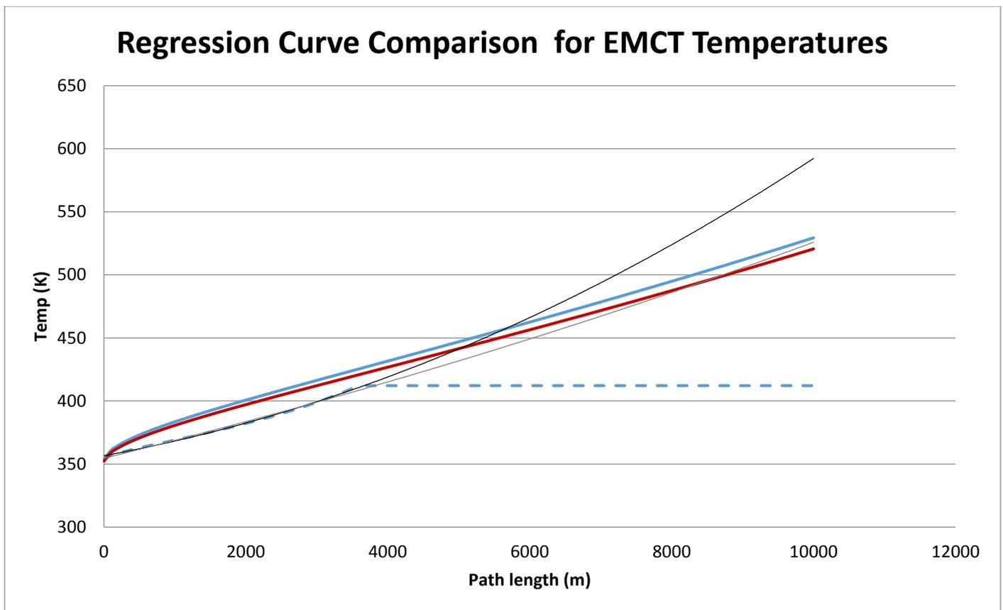
Figure 4 – Comparison of 2<sup>nd</sup> order polynomial regression curve (Ganci et al., 2013) to exponential regression curve: Blue line = temperature calculated using the Planck's method, Red line = temperature calculated using the French et al. (2003) method, Dotted blue line = EMCT temperatures, Black line = Ganci et al. 2<sup>nd</sup> order polynomial regression curve, Grey line = exponential regression curve.
