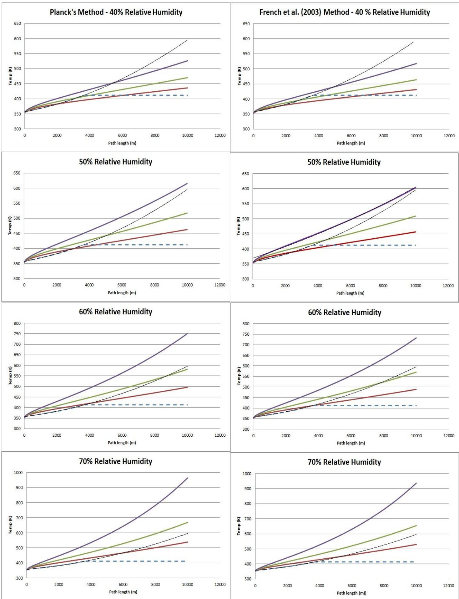
Figure 3 – Comparison of MODTRAN curves with Ganci et al. (2013) regression curve produced using the EMCT temperatures taken at the recorded ambient temperature (21.17 °C) and relative humidity (50.67 %): Dotted blue line = EMCT temperatures, Black line = Ganci et al. (2013) regression curve, Purple line = 25 °C, Green line = 20 °C, Red line = 15 °C.
