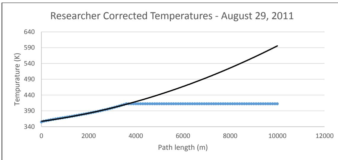
Figure 1 – Regression curve used by Ganci et al. (2013) to extrapolate temperatures beyond the path length correction limit of ThermaCam Researcher: Dotted blue line = EMCT temperatures corrected by Researcher, Black line = 2<sup>nd</sup> order polynomial regression curve used by Ganci et al.
