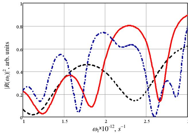
Fig. 2. Reflectance of TM wave incident at  $\Theta_i = 30^\circ$  on the quasiperiodic stack of dielectric layers of thicknesses  $d_1=0.1$  mm,  $d_2=0.07$  mm at  $q=4$  (black dashed curve),  $q=5$  (red solid curve) and  $q=5$  (blue hatched curve) versus frequency
