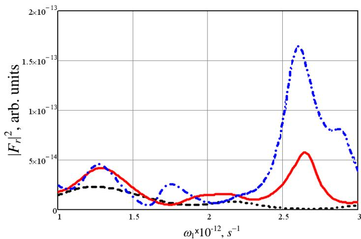
Fig. 3. Intensity of the wave at frequency  $\omega_3$  radiated from the periodic layered structure in the reverse direction of the  $z$ -axis at  $\Theta_{i1} = 30^\circ$ ,  $\Theta_{i2} = 45^\circ$ ;  $\omega_2 = 0.8 \cdot 10^{12} \text{ s}^{-1}$  and  $d_1=0.1$  mm,  $d_2=0.07$  mm at  $q=4$  (black dashed curve),  $q=5$  (red solid curve) and  $q=5$  (blue hatched curve) versus frequency of the first pump wave
