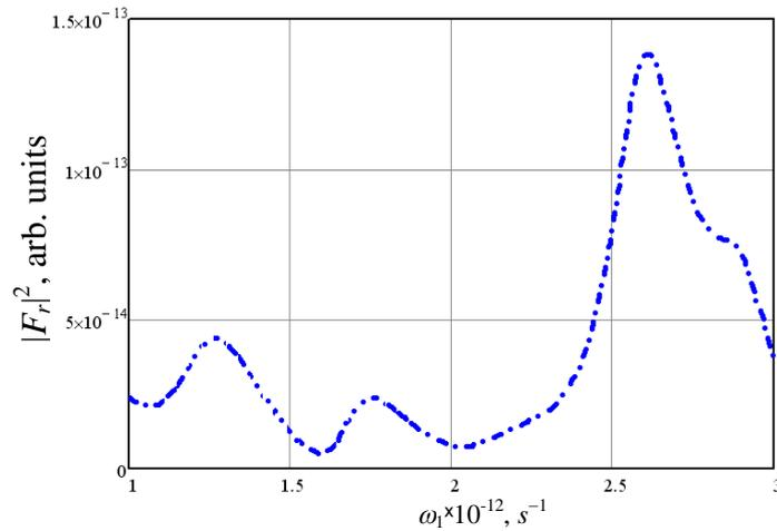
Fig. 4. Intensity of the wave at frequency  $\omega_3$  radiated from the periodic layered structure in the reverse direction of the  $z$ -axis at  $\Theta_{i1} = 30^\circ$ ,  $\Theta_{i2} = 45^\circ$ ;  $\omega_2 = 0.8 \cdot 10^{12} \text{ s}^{-1}$  and  $d_1=0.1 \text{ mm}$ ,  $d_2=0.07 \text{ mm}$  at  $q=6$  and  $\text{tg } \Delta_{xx,zz} = 0.5$  versus frequency of the first pump wave
