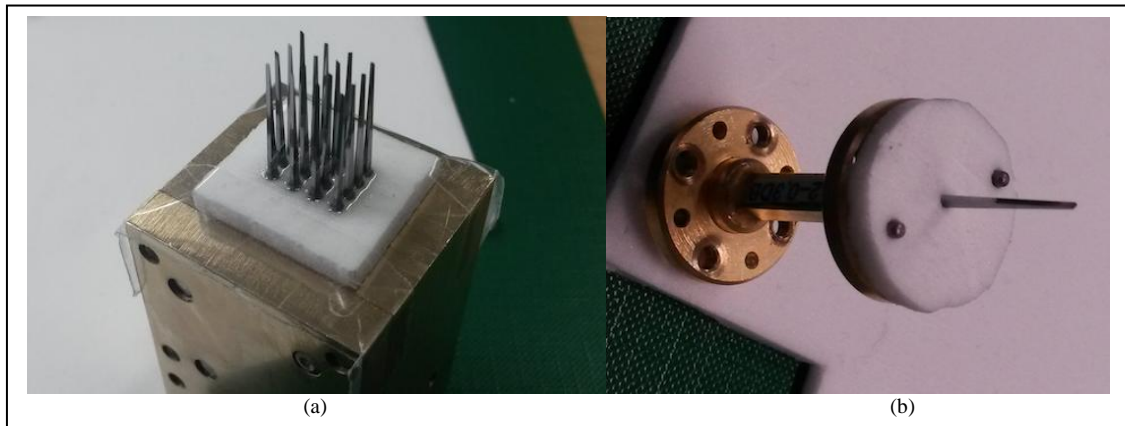
Fig. 4. Manufactured prototypes. Both array (a) and single element (b) DRW antennas were assembled.
