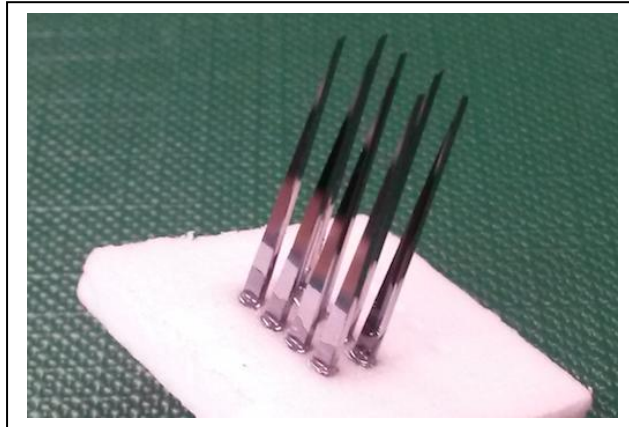
Fig. 3. Assembly of dielectric rod waveguide antennas. They are manually placed in a foam holder, aligned and glued. Two columns are already placed.
