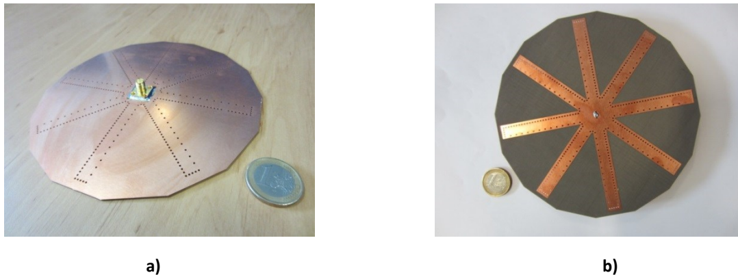
Fig. 2 Detailed view of the feeding of the LWA: a) Rear view and b) top view.
