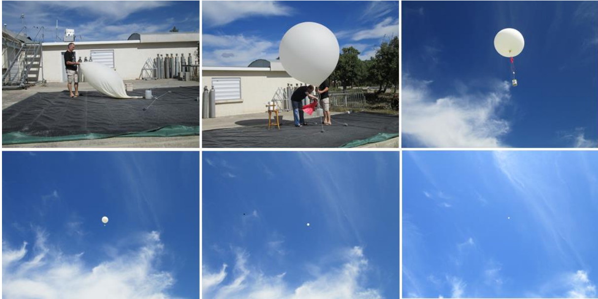
Fig.2. Time series of balloon filling and launching for airborne measurements of ozone concentration in the atmosphere with a balloon at Observatoire de Haute-Provence, France
