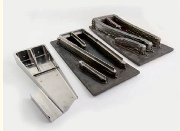
Figure 8. Additively manufactured titanium components for aerospace © Norsk Titanium, Norway
