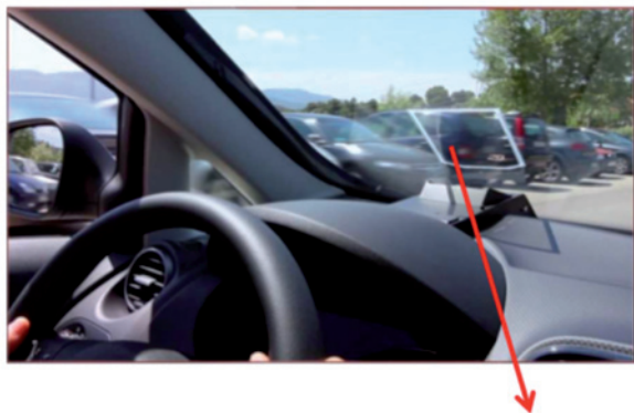
Figure 7. Ultra Thin Metal Film, used for projecting the view from the rear of the car (heads-up display function). Credit: ICFO
