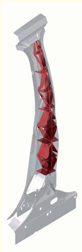
Figure 8. ELiSE procedure (from left to right): i) Planktonic organisms are screened for structures that have similar functions to the given problem, ii) The load cases of the given problem are analysed, iii) the construction methods and archetypes are abstracted, iv) the model is elaborated and further optimised and v) the best solution is referenced to the mechanical problem at hand (in this case, the base of an off-shore platform). Credit: AWI
